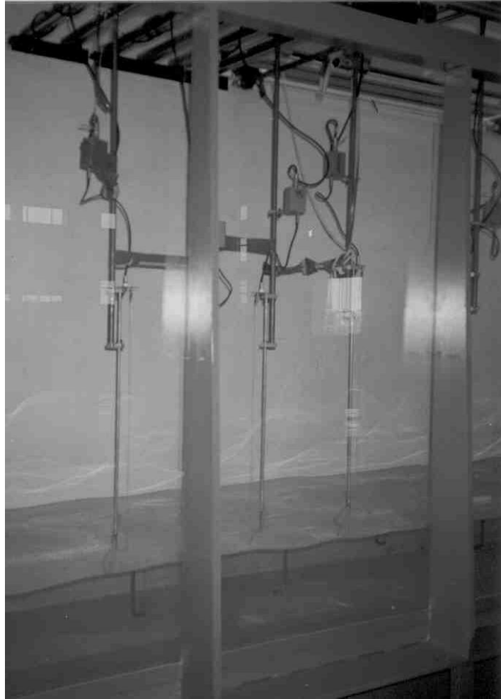
Photo 5. Wave gauges in the flume
